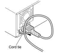
**10. AC INLET** AC power input terminal (3-core)
